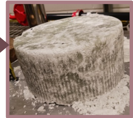
Recovered PP before vacuum drying
